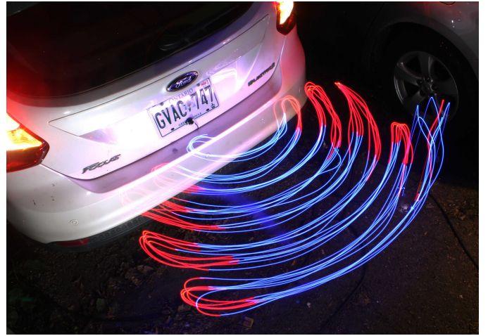
Fig. 8. Metaveillograph of a backup camera captured by the drones flying arcs in a 2D plane.
